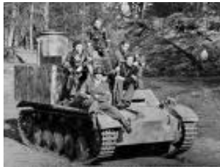
Just like the "coalbed methane" it is common that in "WTC" with a gasifier connected on the back. Commonly based on gasification for most of military needs as it will supplies more fuel all time on the way.
